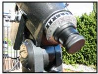
As with other CG-5 clones, the EQ-10 has a nice system for adjusting latitude and azimuth for good polar alignment. The polar alignment scope has a reticule that allows alignment in both hemispheres. Curiously, the focus of the polar scope appears relatively fixed – for persons with 20/20 vision. Take off your glasses, and it's hard to adjust the focus enough to sharpen the images.
