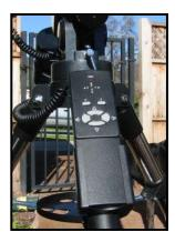
pack and having extra wires dangling around. Speaking of wires, it should be noted that there are only two wires connected to the scope – one runs from the hand controller to the RA motor box. The second runs from the RA motor box to the Dec motor box. The wires are miniature coiled cables, with small plugs reminiscent of a PC's mouse port connector.
