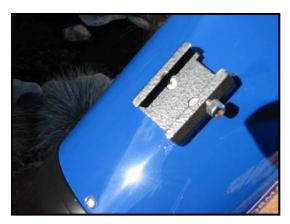
One problem I experienced was the mounting of the finder dovetail. It was not in line with the optical axis, and resulted in making it impossible to align the finder. This problem has been reported by at least two other owners. I found that by loosening the two mounting screws, turning the dovetail slightly, then retightening the screws solved the problem.
