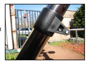
loosening the clamps and moving them upward, you can achieve the proper angle for stability.
