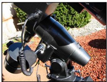
Depending on the ambient temperature, the mount is very stiff when rotating on either axis. At room temperature, it isn't too bad, and if you close your eyes, you can pretend that you are moving a huge observatory telescope on a precision engineered mounting. The stiffness makes the OTA feel smooth and massive. When the temperature gets below 40 degrees, however, things start to get difficult. You have to use two hands to turn each axis. This stiffness is well documented on sites like
