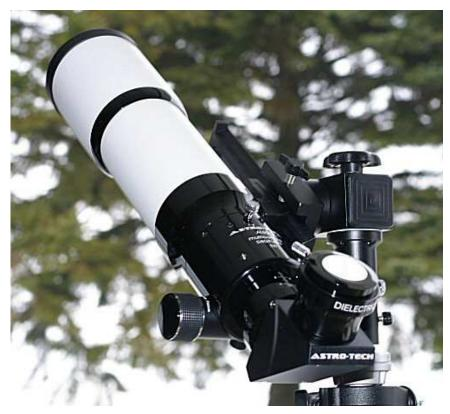
the telescope usually has to be returned for replacement. But with a cemented doublet, if it's collimated, it's going to stay collimated. If it's out – well, Astro-Tech feels confident enough in their products to offer a 2 year warranty.
